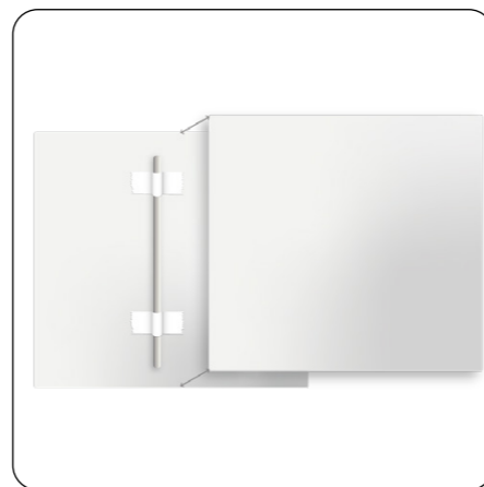
Sandwich lollipop sticks or straws between two pieces of card and glue.
